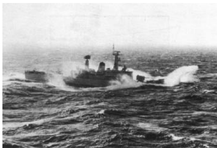
Figure 2- Deck wetness on a frigate, from Lloyd (1989).
