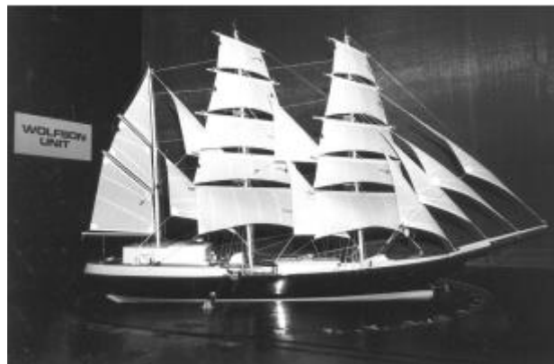
Figure 1 Scale model of the S.V. Tenacious inside the university of Southampton wind tunnel
