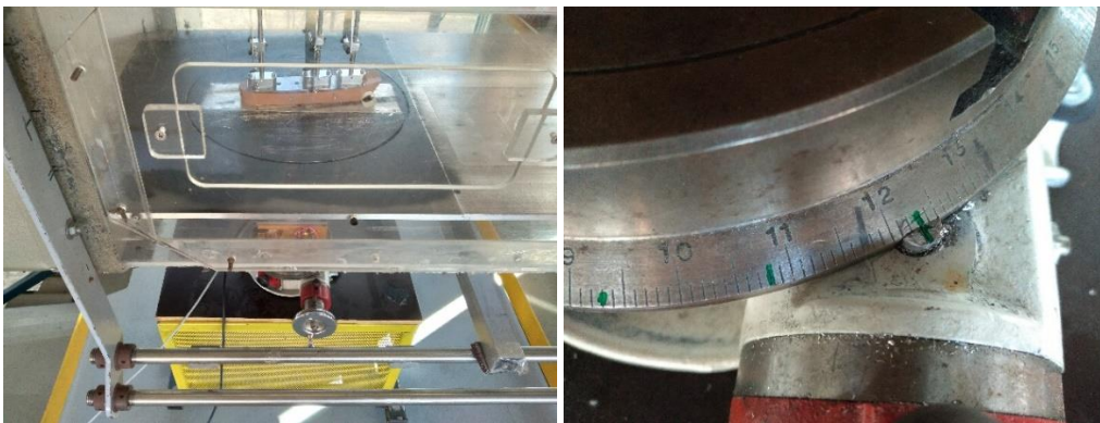
Figure 7 Shows the wind tunnel itself (left) and the turntable (right). For zero-degree AWA drive forces runs, the turntable was set to 123 degrees and 213 degrees for side forces.
