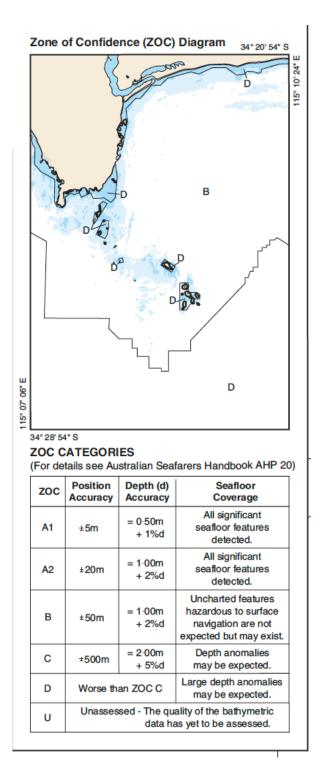
The diagram above is for the Cape Leeuwin/Flinders Bay region and is typical of southwestern WA. The chart area is divided into zones (A, B, C etc.) each with a different level of accuracy. Most of the bay is zone B (position accuracy to + or -50m), which is a lot less accurate than your GPS. The areas where the short cuts past the Cape through the reefs lie is zoned D - accuracy worse than 500m!
