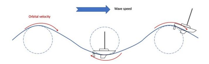
Figure 2: Orbital velocity of wave particles
