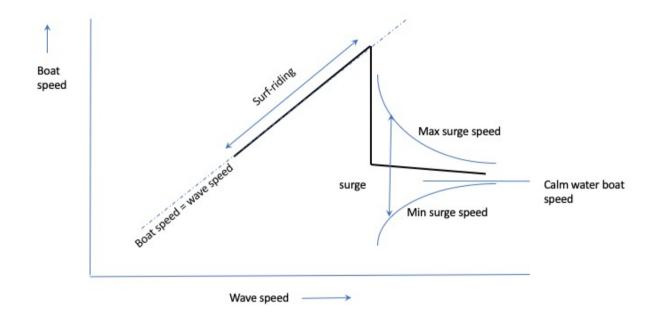
Figure 3: Boat speed in waves (from du Cane and Goodrich)
