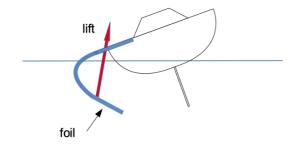
What is a foil trying to do? It is designed to either increase the sail carrying power (righting moment), or lift the hull partially out of the water, or a bit of both. This requires the foil to generate lift force.
