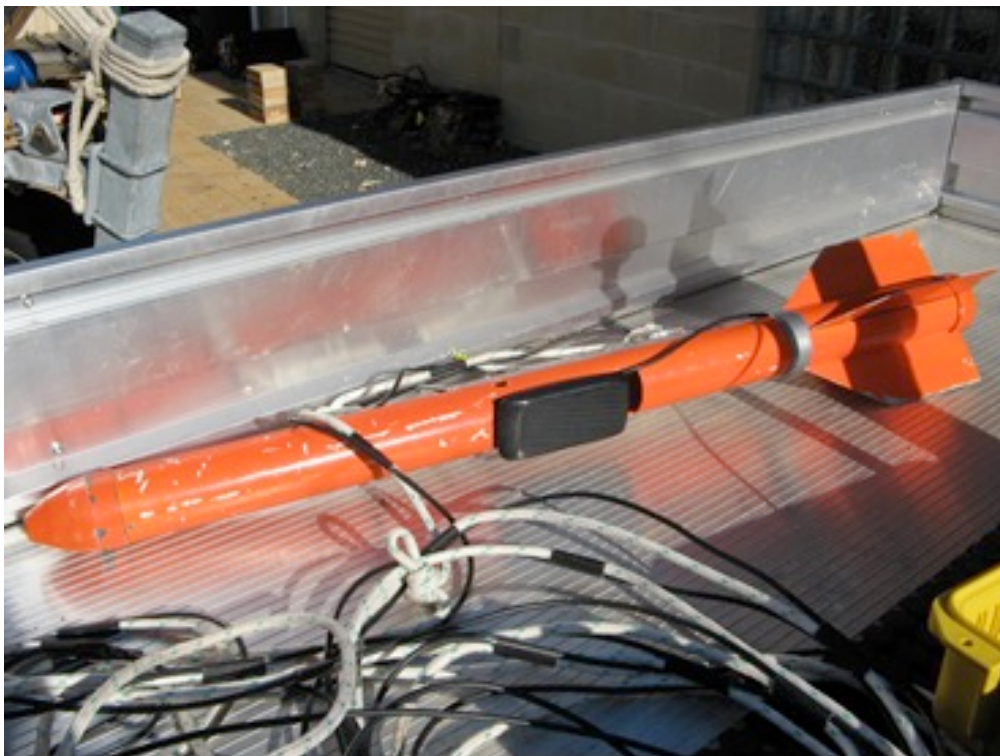
Figure 1 transducer (black) attached to towfish (orange)
