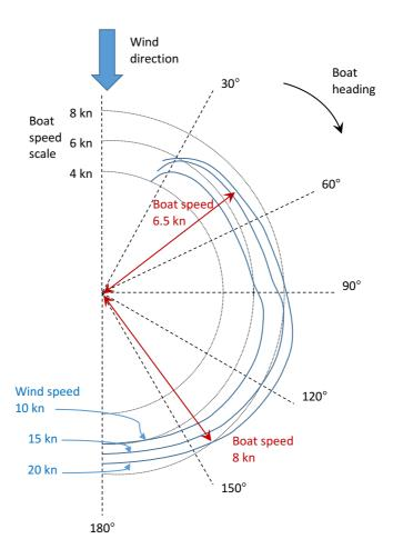
Putting this all together, if you choose a particular wind speed curve, and choose a particular wind angle, then where the curve intersects that angle, its distance from the
