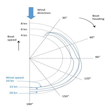
If you already know what a polar plot is, skip to the next section. The polar plot is a very concise way of showing what your boat speed should or could be over a range of wind speeds and wind angles.
