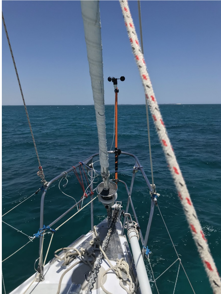
Figure 2: Anemometer deployment and stem head configuration
